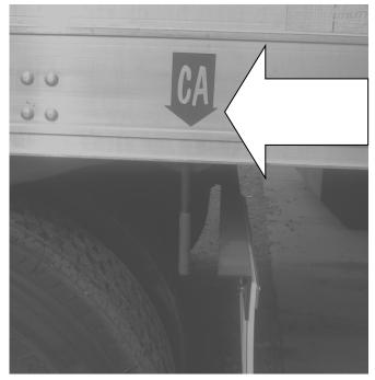
This photo shows where the stop bar needs to be inserted to ensure compliance with the state of California. The arrow points to the holes in the trailer's sub-frame for the stop bar. **NOT** to where the rear of the trailer tire should be or the bracket for the mud flap.
